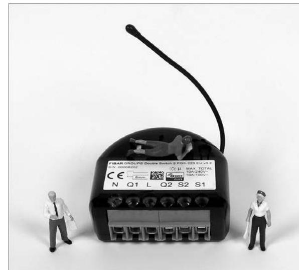
Abbildung 3.20 Fibaro Double-Switch FGS-223
